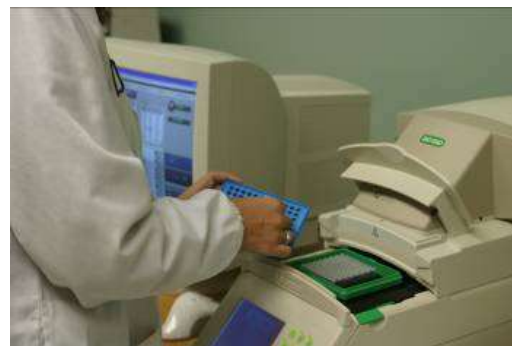
6) PCR amplify specific genes (e.g., 16S rRNA/ vcrA ) with targeted primers in qPCR Machine
