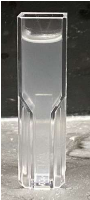
Photo of processed O/W emulsion after 1 hour
