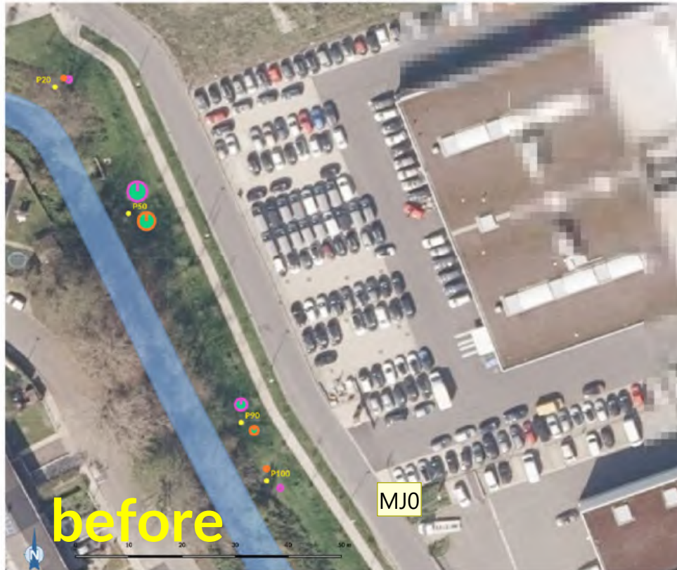
Horizontal Mass Fluxes: Before Dredging
